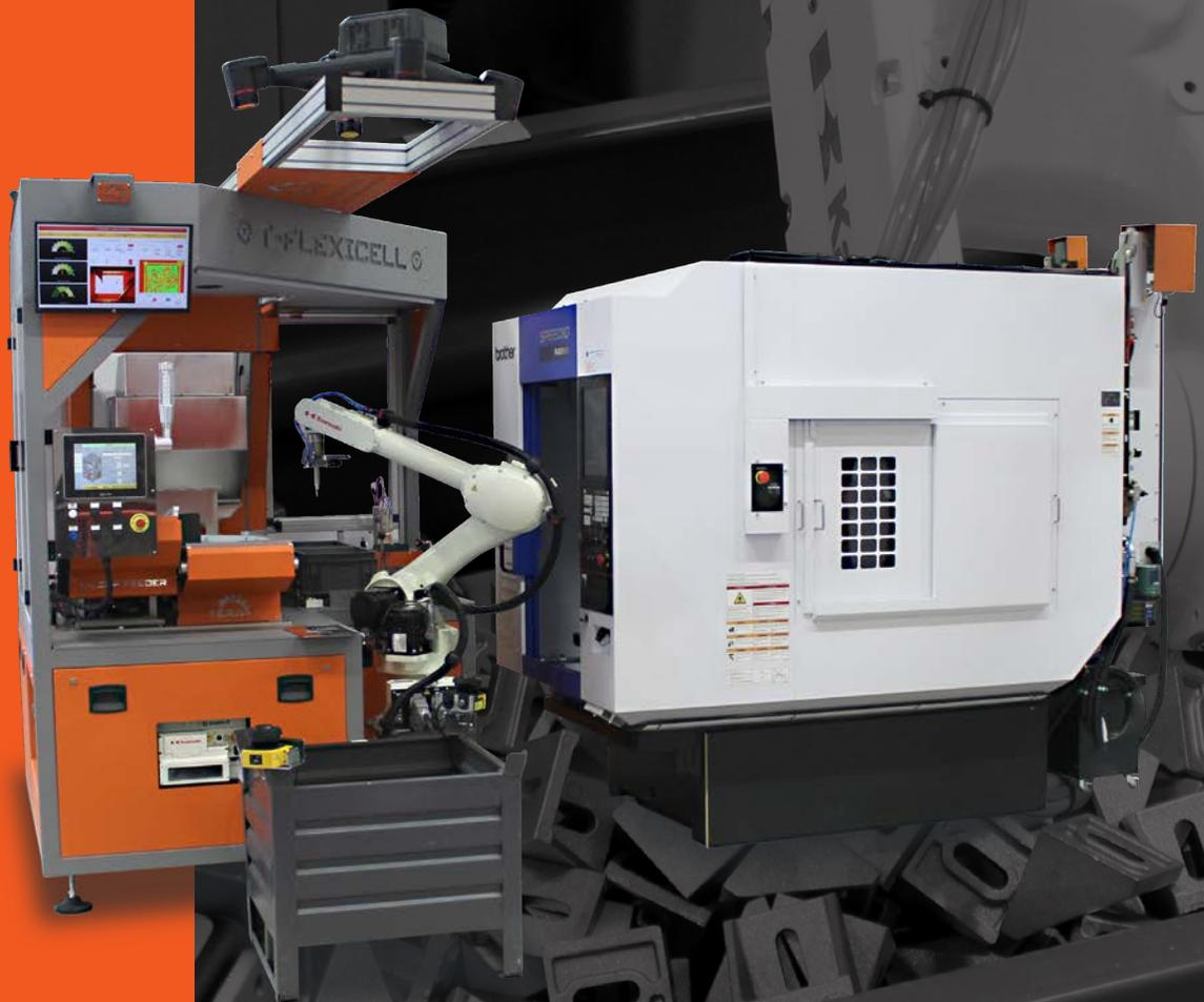
**Robotic cell for CNC machine tending**
