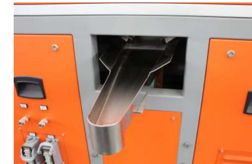
Outlet vibrating channel
