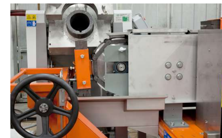
Tilting furnace + Mold ready for vertical casting
