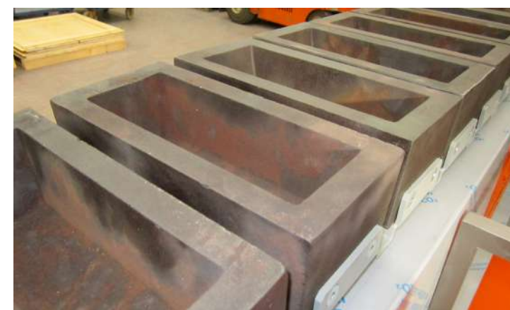
Molds for bars casting
